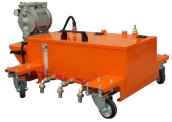
The *Recovery Filtering Unit* collects the unused fluid from the Suction System and the Spray Chamber. Three filters separate the emulsion fluid from the protection fluid that, once filtered, is brought automatically to the main tank, ready to be reused.
