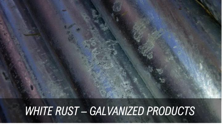
Storing pipes & profiles without sufficient Rust Prevention Oil (RPO) will result in rust formation and consequently huge claims for the poor quality of the end products that could be rejected from end customers.
