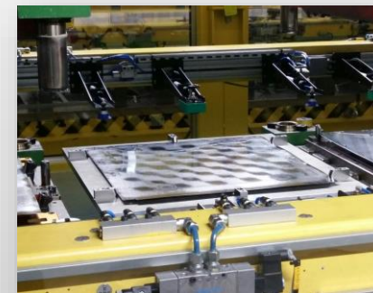
Sectorial lubrication in squares 50x50 mm
