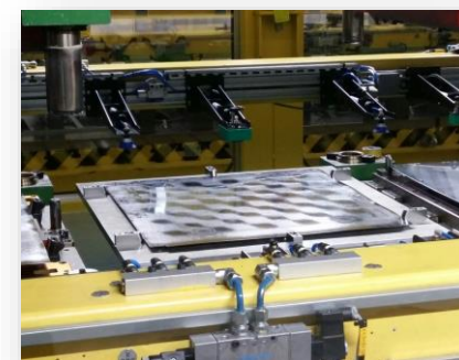
Sectorial lubrication in squares 50x50 mm
